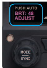
Figure 5-26 Display Brightness in BRT ADJUST Mode
