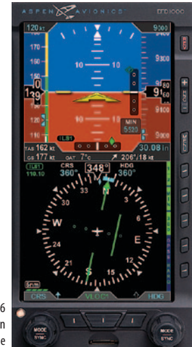
Figure 3-36 Vertical and Horizontal Deviation Indicator, Showing Glide Slope
