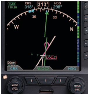
Figure 4-41 ARC HSI Compass Mode
