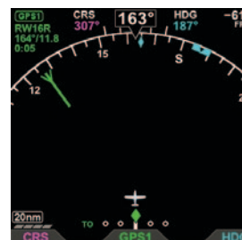
Figure 4-51 Stub Course Tail, ARC CDI Compass Mode
