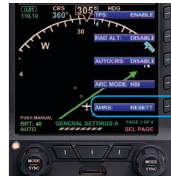
Figure 6-7 AHRS Reset Menu Key
