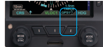
Figure 4-81 Double-Line Bearing Pointer and Button
