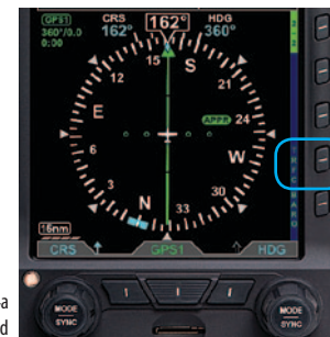
Figure 4-114a Traffic Overlay Disabled
