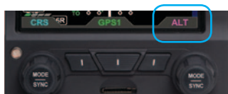
Figure 3-19 Altitude Field Enabled
