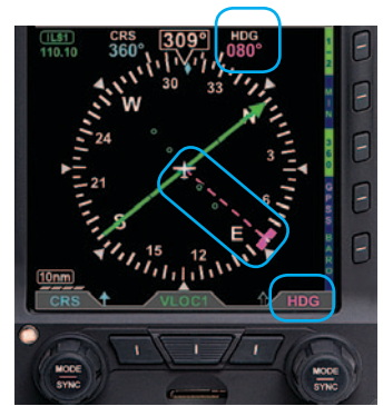
Figure 3-8 Selected Heading Field Enabled
