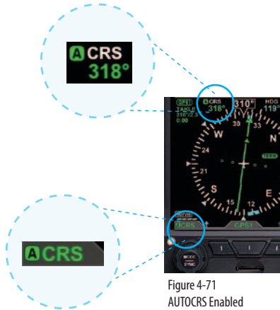
Figure 4-70 AUTO CRS Enabled
