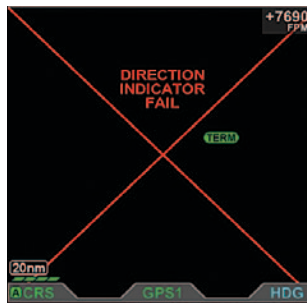
Figure 4-86 Direction Indicator Fail
