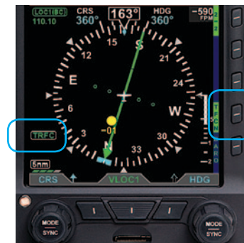
Figure 3-17 Traffic Overlay On
