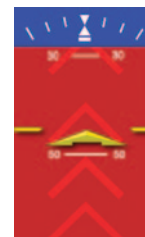
Figure 4-5 Pitch Markings - Chevrons indicate Pitch Up
