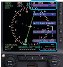
Figure 4-20 BARO Set to mB (millibars)
