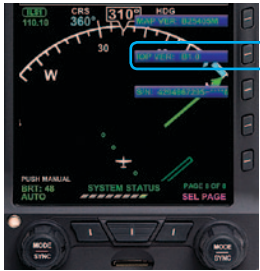
Figure 7-2 View Input/Output Processor Software Version
