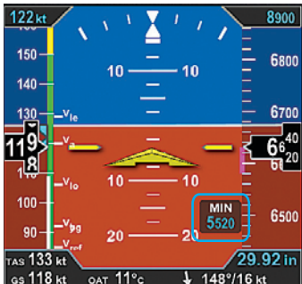
Figure 4-29 Selected MINIMUMS Annunciation and Markers Enabled
