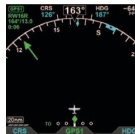
Figure 4-50 Stub Course Arrowhead, ARC CDI Compass Mode
