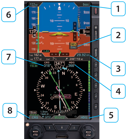
Figure 2-3 Left and Right Knobs and Corresponding Fields
