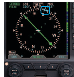
Figure 4-82 Heading Bug and Selected Heading Field
