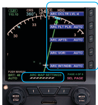
Figure 5-10 ARC Compass Mode Display Options
