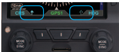
Figure 3-12 No Bearing Pointer Sources Selected
