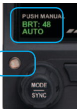
Figure 5-25 Display Brightness in BRT AUTO Mode
