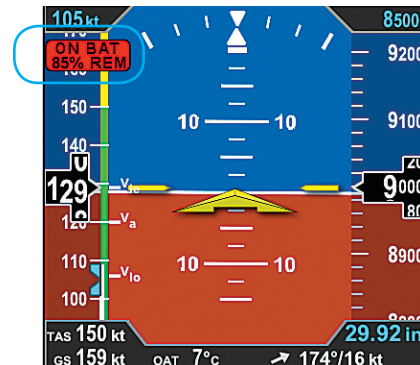
Figure 6-2 Battery Charge Remaining
