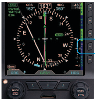
Figure 4-111 GPSS Disabled and Autopilot in HDG Mode
