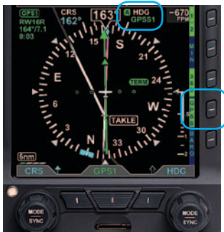
Figure 4-110 GPSS Enabled with Autopilot in HDG Mode
