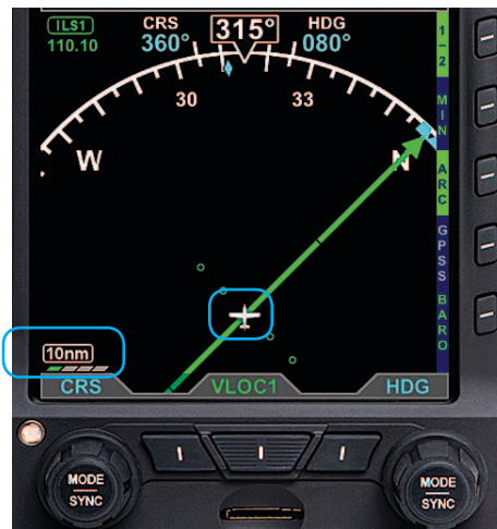
Figure 3-16 Current Range 10nm from Ownship to Edge of Compass Rose
