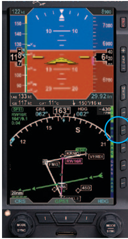
Figure 4-28 MIN Hot Key – Selected MINIMUMS Annunciation and Markers Disabled
