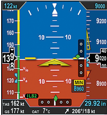
Figure 2-32 Instrument Approach Indications
