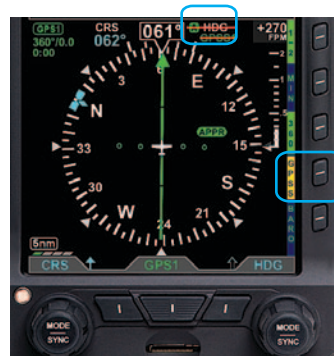
Figure 6-10 GPSS in Wings Level Mode
