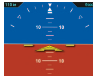
Figure 4-13 Airspeed Tape Disabled
