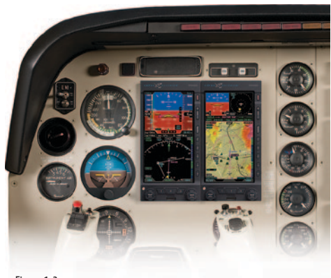
Figure 1-3 Dual Display System: PFD & MFD
