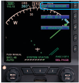
Figure 7-1 View Main Application Processor Software Version
