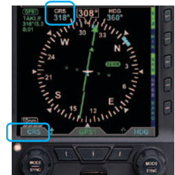
Figure 4-75 CRS Field Enabled for Editing
