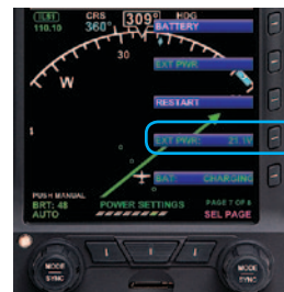
Figure 6-3 External Power Voltage Status
