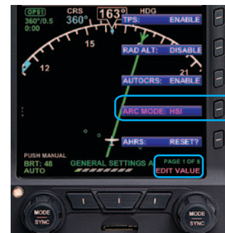
Figure 4-44 Changing the ARC Compass MODE
