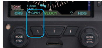
Figure 4-80 Single-Line Bearing Pointer and Button
