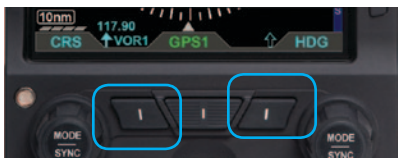
Figure 3-11 Bearing Pointer Nav Source Select Buttons
