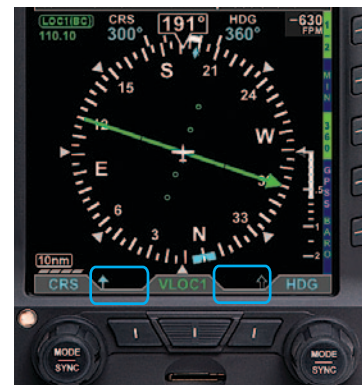
Figure 4-77 Bearing Pointers OFF
