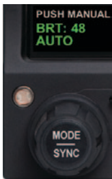
Figure 2-24 Display Brightness in BRT AUTO Mode
