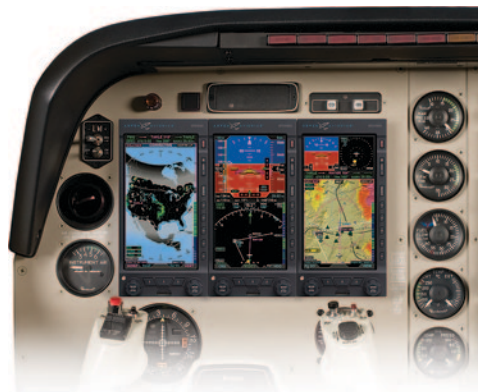
Figure 1-4 Trio Display System: PFD & Dual MFDs
