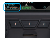
Figure 4-78 Invalid Bearing Pointer Source
