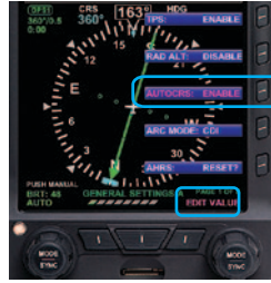
Figure 4-70 AUTO CRS Enabled
