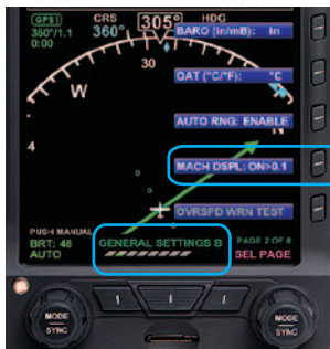
Figure 4-13b Speed Transition Setting
