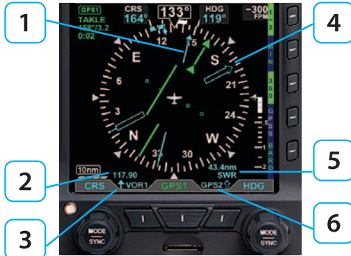
Figure 4-76 Bearing Pointer Description
