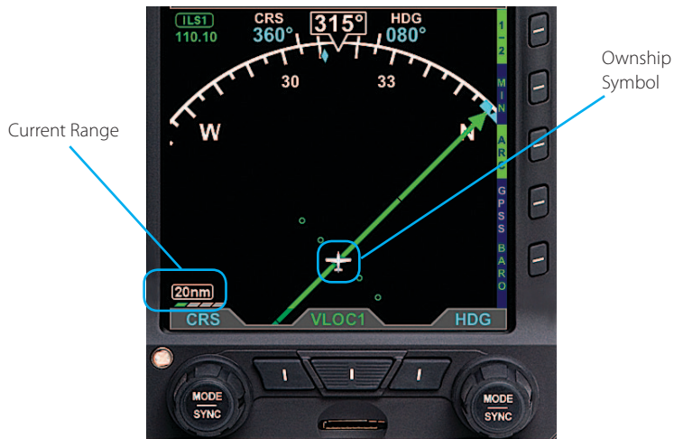
Figure 3-15 Current Range 20nm from Ownship to Edge of Compass Rose
