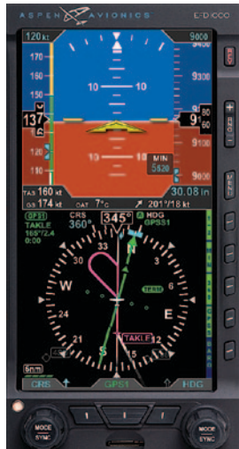
Figure 3-35 360° Mode Showing Procedure Turn, GPSS Enabled
