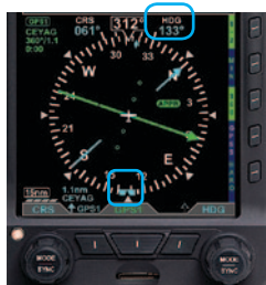
Figure 2-6 HDG field updated and inactive
